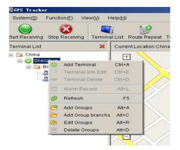
4.26. Terminal Management: Select an established terminal from the Terminal List drop-down list box and then click the right button. Users are allowed to modify the terminal/check out alarm records/add or remove terminals etc. as shown below:
