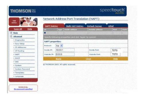
4.7.5.4 Select the TCP mode and then enter 10.0.0.1 into the column of Internal IP that is identical to that in the PC. Type in 7070 into the fields in connection with Inside Port and Outside Port respectively.
